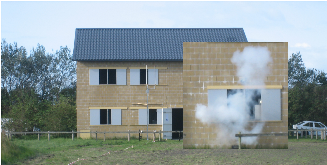
Figure 6-16: RUAG Generator for Flash Sound and Smoke.
